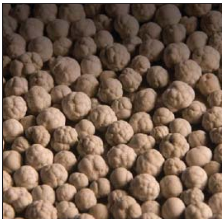
Struvite, a combination of minerals from thin stillage can cause trouble for digesters, but could have value as fertilizer.
