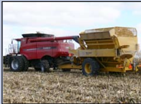
This pull-type cob collection system was one of two harvest technologies tested.
